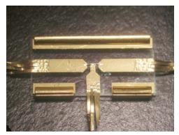
The mixer diodes themselves are almost too small to see, even in the magnified view at bottom. Actual width of the entire substrate is approximately 15 mm.
