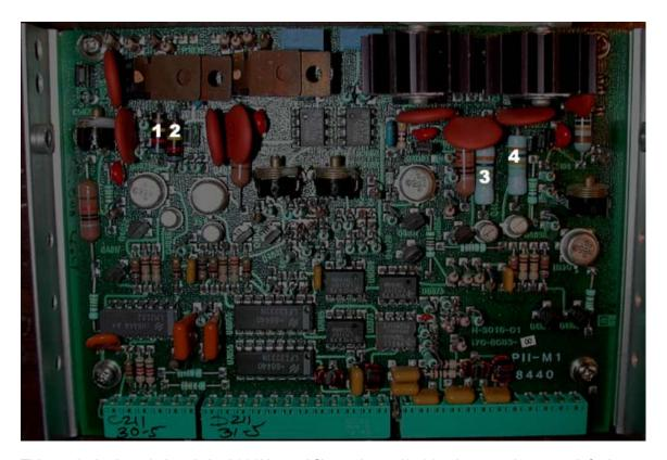
This particular board already had 300K metal film resistors (3,4) in place, so they were left alone. The 620K, 5% carbon-composition resistors (1,2) were measured at 580K and 980K, respectively.
